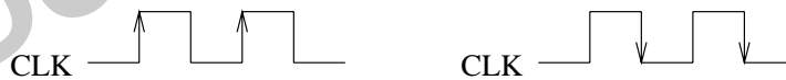
Figure 18: Clocks in timing diagrams for positive-edge triggered (left) and negative-edge triggered (right) devices.
